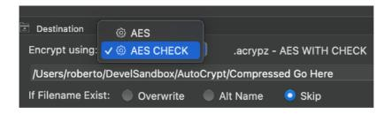
Suggested method is AES CHECK. It is very very strong, it uses a 256 bit key and a random password salt and a random initialization vector. If you encrypt the same file for 2 different times using the same password, the 2 encrypted file will be different, but still decryptable using the correct password. It includes a check to verify if the password used is the correct one.
