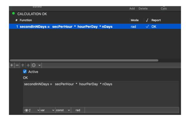
It is self explanatory, to calculate the seconds in a week we calculated the seconds in 1 hour multiplied per hours in one day multiplied the nDays value
