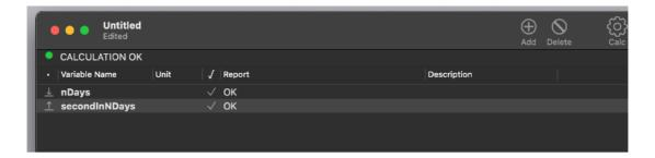
With 'Auto insert Variables' not only TS Calc realised we inserted two new variables not yet defined but it also recognised one is used as input and the other as output. As you can see they have 2 different icons marking them inside the variable table
