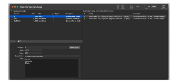
When the automatic feature to add variable used inside an equation is used, the user has to manually move a variable to the constant area if it has to be managed as a constant, the application has no way to know it in advance.
