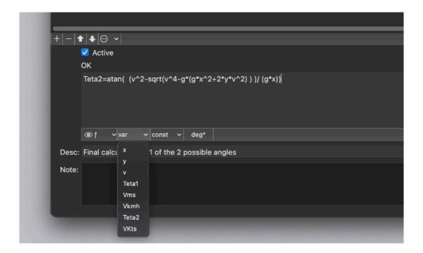
constants and functions available to put inside the functions and a fourth button 'Autoinsert Variables <<' used to recognize new variables, inserted in the body of the function, and to add them in the Variables View )
