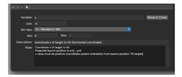
A variable name to be acceptable must be alphanumeric, start with a letter and with no space inside, the only non alphanumeric acceptable char is '\_'
